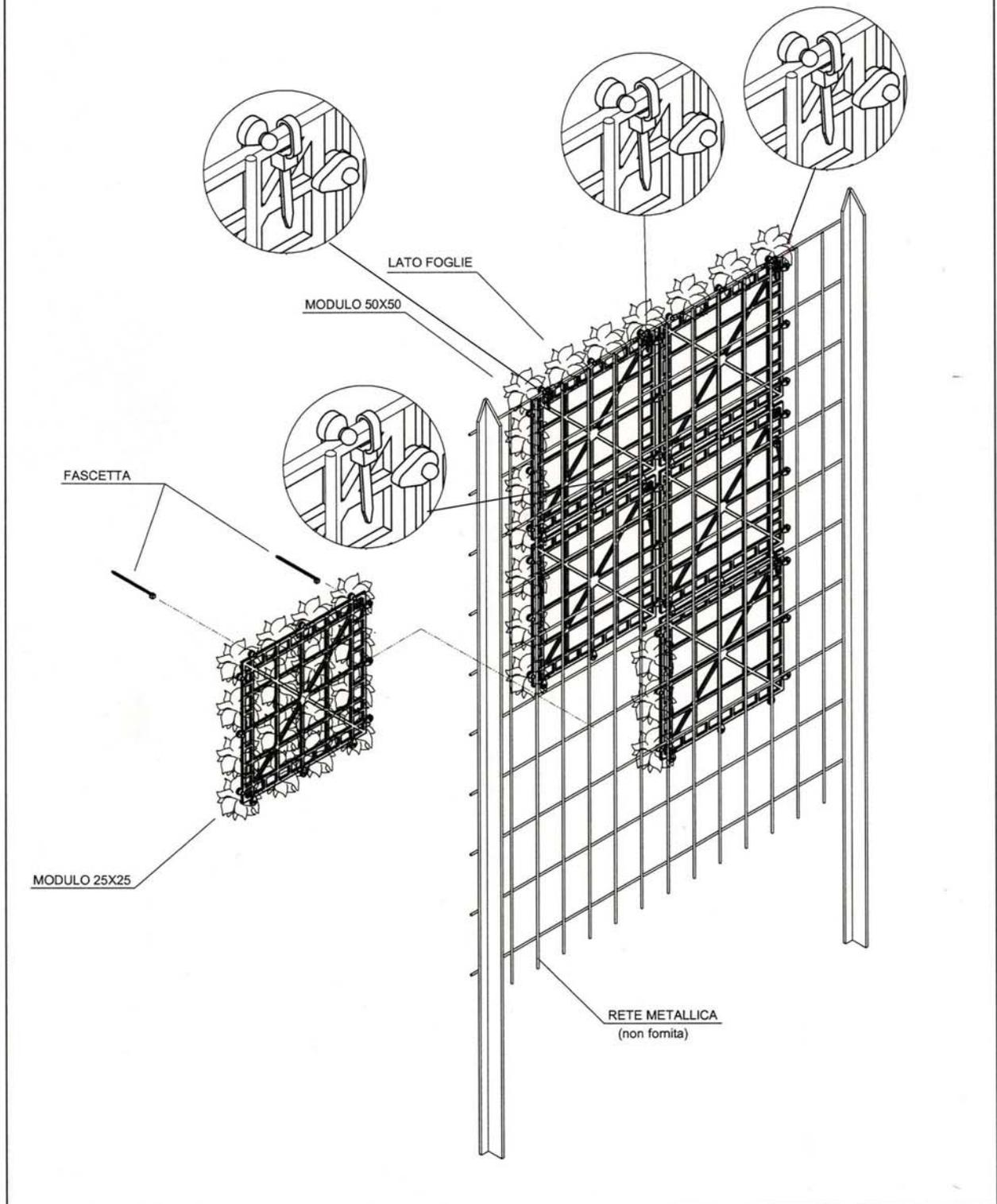
SCHEMA MONTAGGIO/SMONTAGGIO MODULI E SOTTOMODULI
